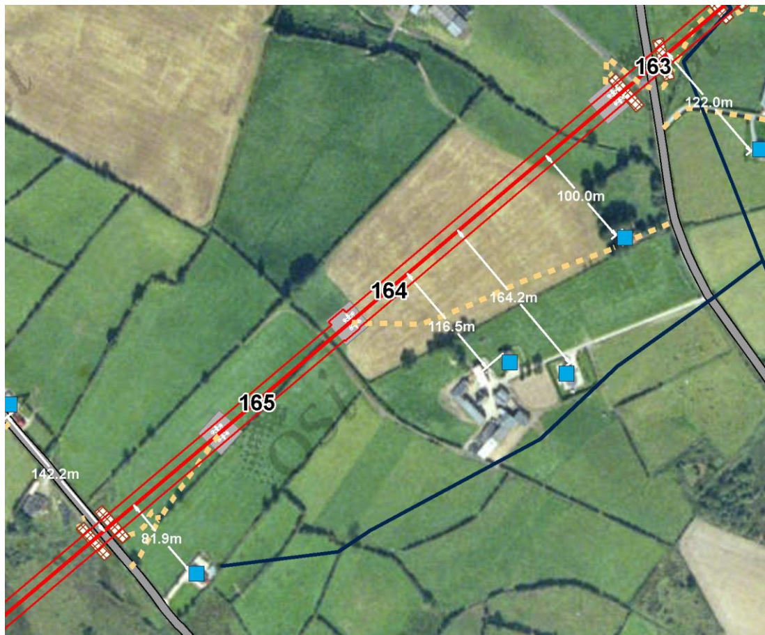
Figure 7.3: Illustration of excavation necessary at Tower 164
